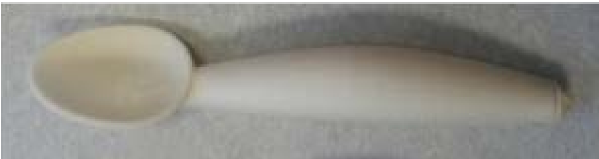
Figure 3 –The two-piece plastic SOUP Spoon made using 3D printing.
